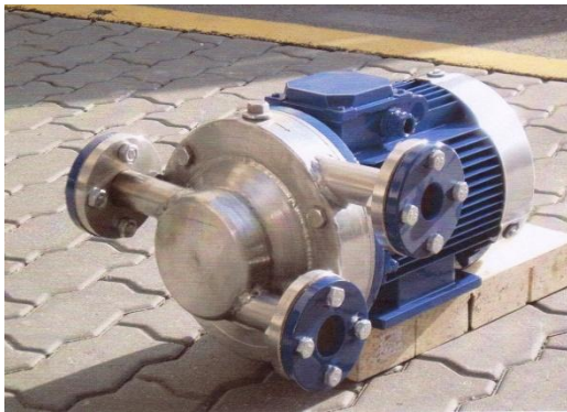
Figure 7. High-speed mixer-disperser DRS10 (capacity -10 m 3 /h, pressure - 0.2 MPa, motor power - 5,5 kW)
